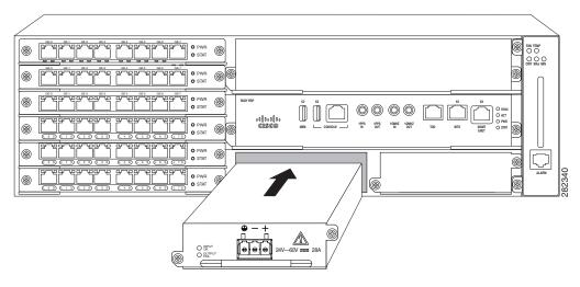
Figure 3-16 Installing the DC Power Supply
